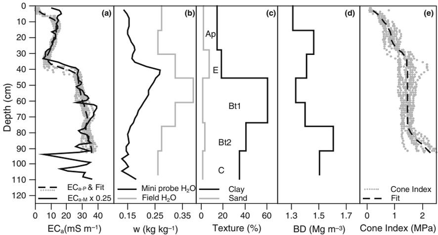
**Fig. 19.1** Data from a representative claypan soil on field A. (a) Penetrometer electrical conductivity ( $EC_{a-P}$ ) and scaled Wenner mini-probe conductivity ( $EC_{a-M} \times 0.25$ ). (b) Field (taken with  $EC_{a-P}$ ) and high-resolution (taken with  $EC_{a-M}$ ) gravimetric soil moisture ( $w$ ). (c) Percent clay and sand. (d) Bulk density (BD). (e) Cone index
