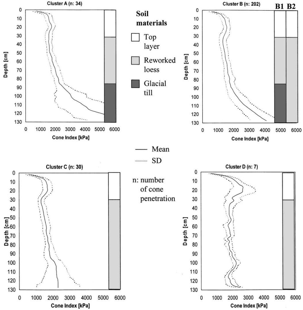
Fig. 4. CIPs and soil materials for cluster A–D. Depths where cone penetration resistance are significantly different at the 0.05 level are indicated with the same letter; those with no significant differences are not listed.
