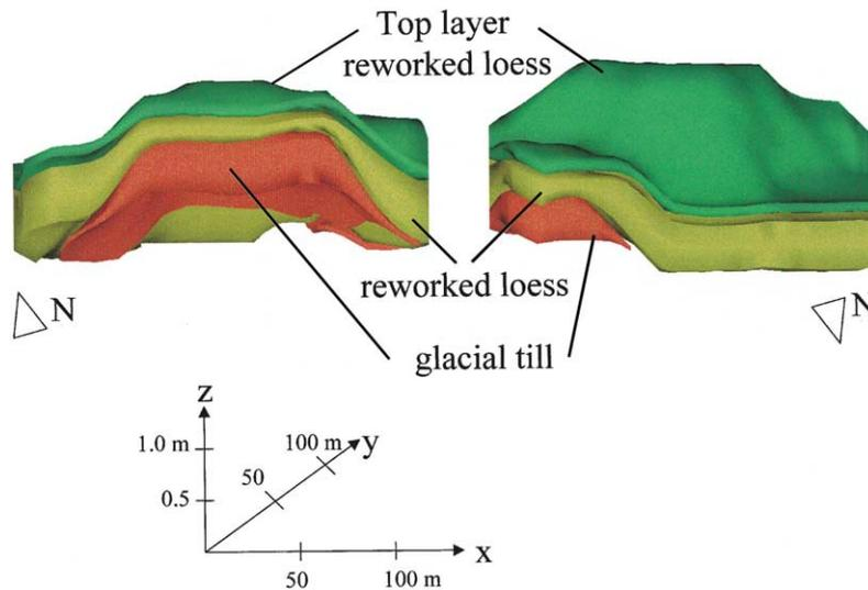
Fig. 6. Three-dimensional soil layer model showing the spatial distribution of soil materials.
