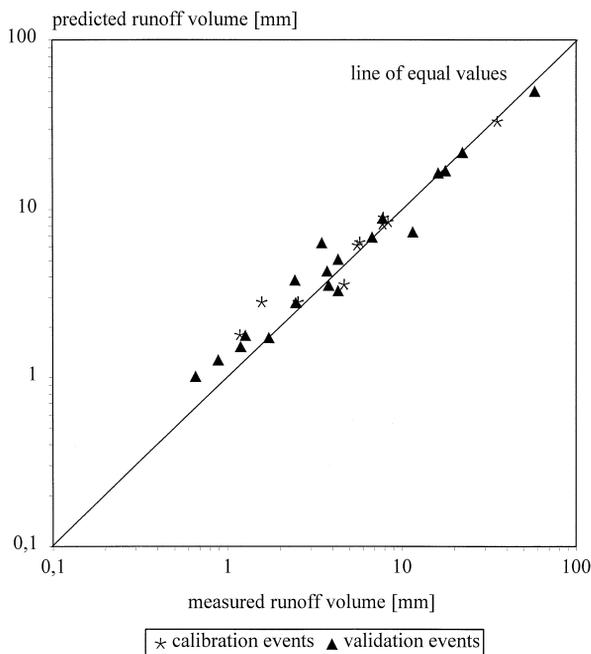
Fig. 1. Measured and predicted runoff volume—Glonn G1 watershed.
